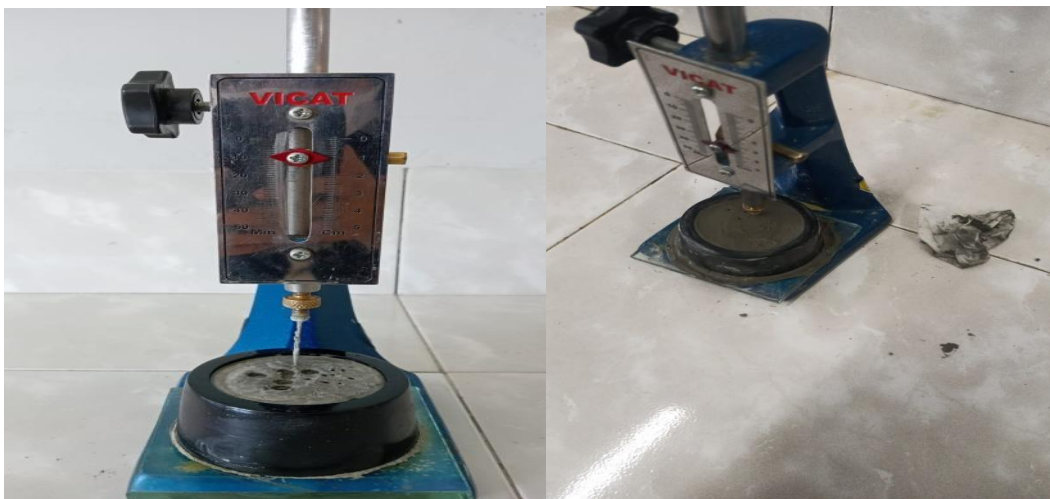
Gambar 4.4 Pengujian setting Time
